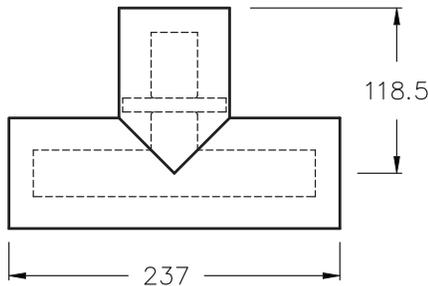
Tee assembly, unflanged, copper construction. Includes only supported inner conductor.
