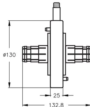
Gas barrier with silicone O-ring and stainless steel hardware set.
