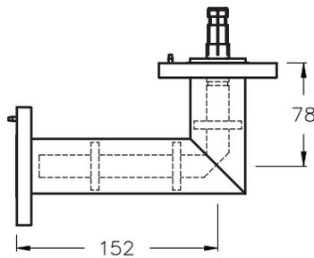
Miter elbow 90°-unequal legs, swivel EIA flanges on both ends, brass and copper construction. Includes supported inner conductor, one anchor insulator conductor connector, silicone O-ring and stainless steel hardware set.
