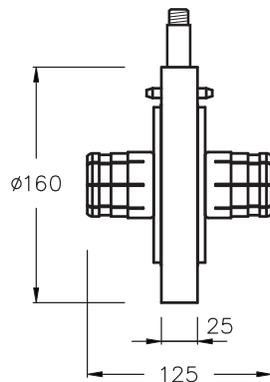
Gas barrier with silicone O-ring and stainless steel hardware set.
