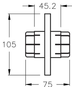
Anchor insulator conductor connector, for EIA flange connection, silver plated. **Short version.**
