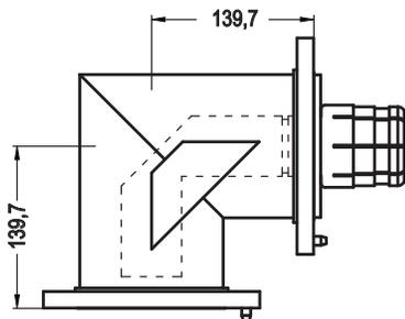
Miter elbow 90°, swivel EIA flanges on both ends, reinforced outside, brass and copper construction. Includes unsupported inner conductor, one anchor insulator conductor connector, silicone O-ring and stainless steel hardware set.
