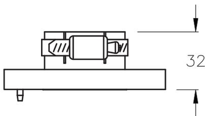
Unpressurized EIA field flange for indoor use. Includes one stainless steel hose clamp and hardware set.
