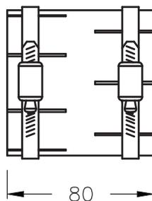
Line coupling for connection of unflanged lines. No inner conductor connector. Includes two stainless steel hose clamps (does not increase outer conductor length).
