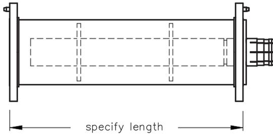
Line assembly, flanged with fixed and swivel flange. Brass and copper construction. Includes one anchor insulator conductor connector, silicone O-ring and stainless steel hardware set.
