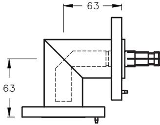
Miter elbow 90°, swivel EIA flanges on both ends, brass and copper construction. Includes unsupported inner conductor, one anchor insulator conductor connector, silicone O-ring and stainless steel hardware set.
