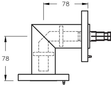
Miter elbow 90°, swivel EIA flanges on both ends, brass and copper construction. Includes supported inner conductor, anchor insulator conductor connector, silicone O-ring and stainless steel hardware set.
