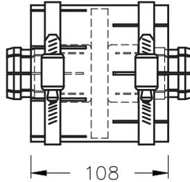
Line coupling for connection of unflanged lines. Includes supported inner conductor connector and two stainless steel hose clamps.
