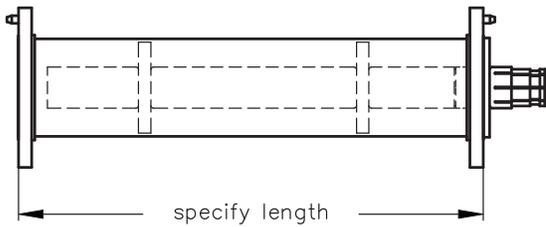
Line assembly, flanged with fixed and swivel flange. Brass and copper construction. Includes one anchor insulator conductor connector, silicone O-ring and stainless steel hardware set.
