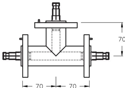
Tee assembly, swivel EIA flanges. Includes three anchor insulator connectors, O-rings and hardware sets.
