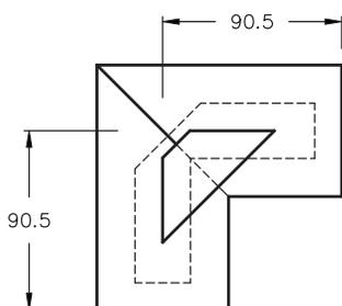
Miter elbow 90°-unflanged, reinforced outside, copper construction. Includes only one unsupported inner conductor.
