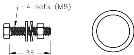
Stainless steel hardware set with silicone rubber O-ring.
