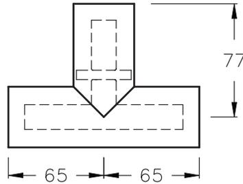
Tee assembly, unflanged, copper construction. Includes only supported inner conductor.
