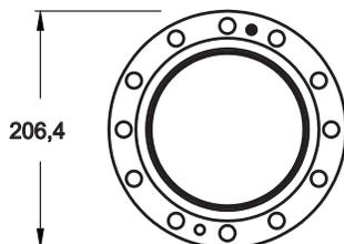
Fixed EIA flange with silver solder ring insert for silver brazing to outer conducting tubing.
