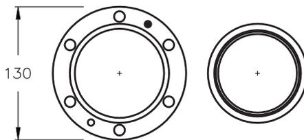
Swivel EIA flange, brass. Includes only sliding and fixed ring prepared for silver brazing to outer conducting tubing.
