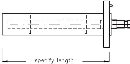
Line assembly, one end fixed flanged. Includes one anchor insulator conductor connector, silicone O-ring and stainless steel hardware set.
