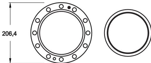
Swivel EIA flange, brass. Includes only sliding and fixed ring prepared for silver brazing to outer conducting tubing.
