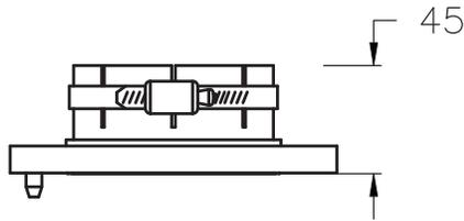
Unpressurized EIA field flange for indoor use. Includes one stainless steel hose clamp and hardware set.
