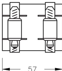
Line coupling for connection of unflanged lines. No inner conductor connector. Includes two stainless steel hose clamps (does not increase outer conductor length).
