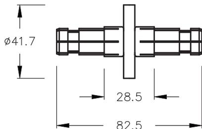
Anchor insulator conductor connector, for EIA flange connection, silver plated. **Standard length.**
