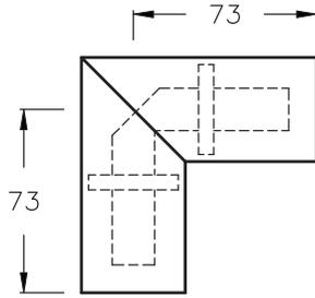
Miter elbow 90°-unflanged, long legs, copper construction. Includes only one supported inner conductor.
