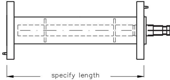
Line assembly, flanged with fixed and swivel flange. Brass and copper construction. Includes one anchor insulator conductor connector, silicone O-ring and stainless steel hardware set.
