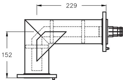
Miter elbow 90°-unequal legs, swivel EIA flanges on both ends, reinforced outside, brass and copper construction. Includes supported inner conductor, one anchor insulator conductor connector, silicone O-ring and stainless steel hardware set.
