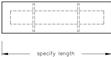
Line assembly, unflanged, no insulator conductor connector or hardware.
