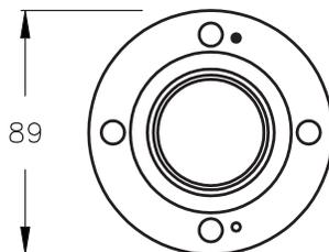
Fixed EIA flange prepared for silver brazing to outer conducting tubing.
