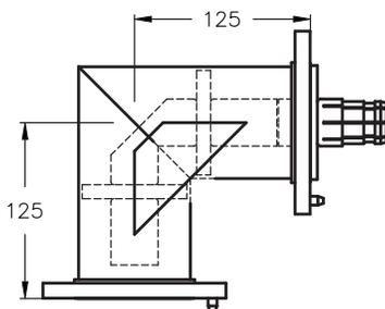
Miter elbow 90°, swivel EIA flanges on both ends, reinforced outside, brass and copper construction. Includes supported inner conductor, anchor insulator conductor connector, silicone O-ring and stainless steel hardware set.
