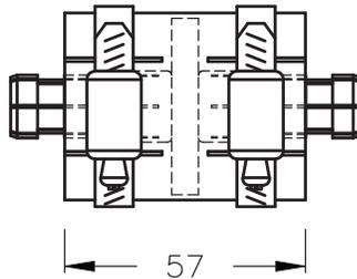
Line coupling for connection of unflanged lines. Includes supported inner conductor connector and two stainless steel hose clamps.
