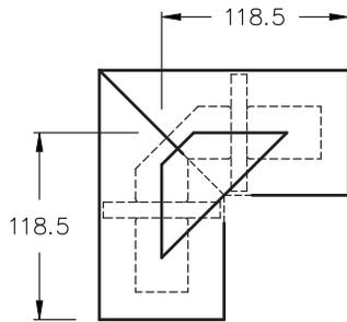
Miter elbow 90°-unflanged, long legs, reinforced outside, copper construction. Includes only one supported inner conductor.
