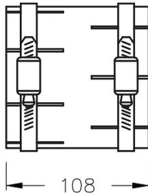
Line coupling for connection of unflanged lines. No inner conductor connector. Includes two stainless steel hose clamps (does not increase outer conductor length).
