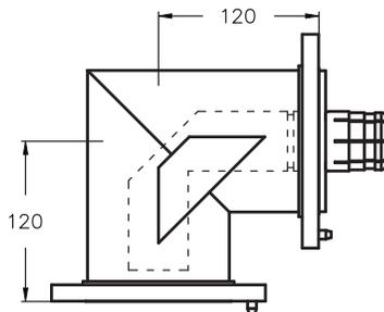
Miter elbow 90°, swivel EIA flanges on both ends, reinforced outside, brass and copper construction. Includes unsupported inner conductor, one anchor insulator conductor connector, silicone O-ring and stainless steel hardware set.
