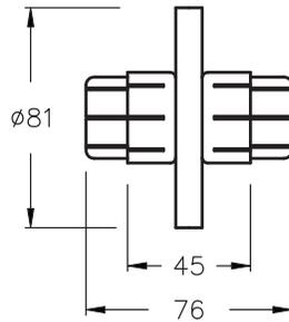
Anchor insulator conductor connector, for EIA flange connection, silver plated. **Short version.**
