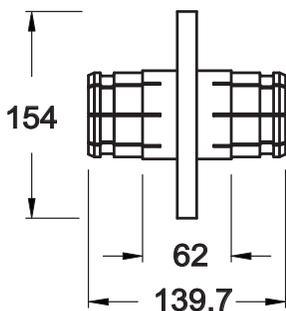
Anchor insulator conductor connector, for EIA flange connection, silver plated. **Standard length.**
