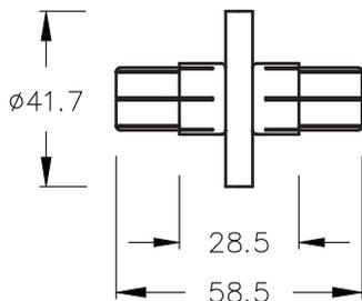
Anchor insulator conductor connector, for EIA flange connection, silver plated. **Short version.**
