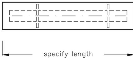
Line assembly, unflanged, no insulator conductor connector or hardware.
