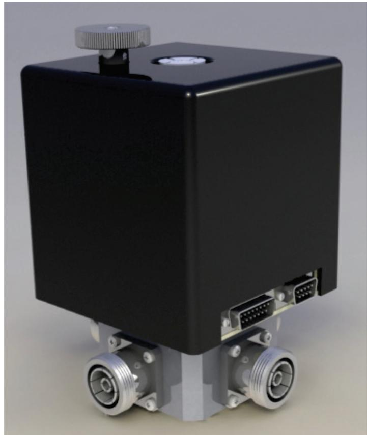
The models SW 716.01, SW 716.02 and SW 716.03 are motor-driven, two-way coaxial transfer switches designed to change coaxial connections with a minimum off-air-time. Mainly they are used for switching transmitters, antennas, dummy loads and other peripheral equipment in situations when broadcasting procedures are modified, when there is need for emergency repair, or during scheduled maintenance.
