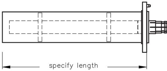
Line assembly, one end fixed flanged. Includes one anchor insulator conductor connector, silicone O-ring and stainless steel hardware set.
