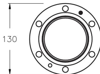
Fixed EIA flange with silver solder ring insert for silver brazing to outer conducting tubing.
