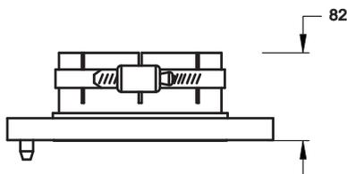
Unpressurized EIA field flange for indoor use. Includes one stainless steel hose clamp and hardware set.
