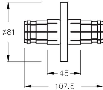
Anchor insulator conductor connector, for EIA flange connection, silver plated. **Standard length.**
