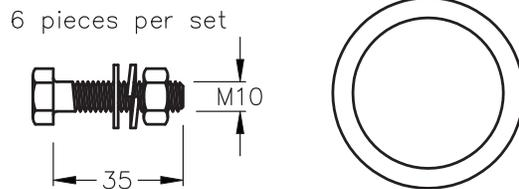
Stainless steel hardware set with silicone rubber O-ring.
