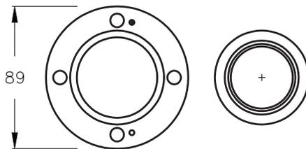
Swivel EIA flange, brass. Includes only sliding and fixed ring prepared for silver brazing to outer conducting tubing.
