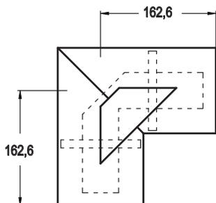
Miter elbow 90°-unflanged, long legs, reinforced outside, copper construction. Includes only one supported inner conductor.
